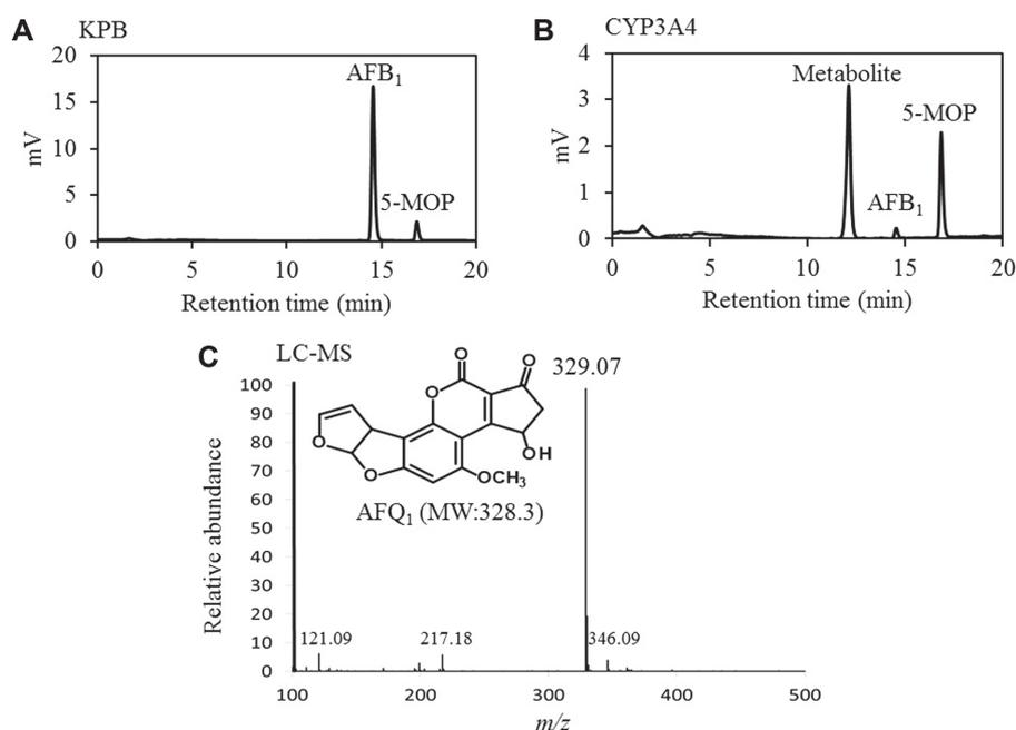
**Fig. 3. Metabolite identification by LC-MS.** We conducted metabolic experiments using *E. coli* expressing human CYP3A4 and analyzed the metabolites by HPLC. (A) KPB, (B) CYP3A4. (C) The peak of the metabolite obtained in (B) was collected and identified by LC-MS.
