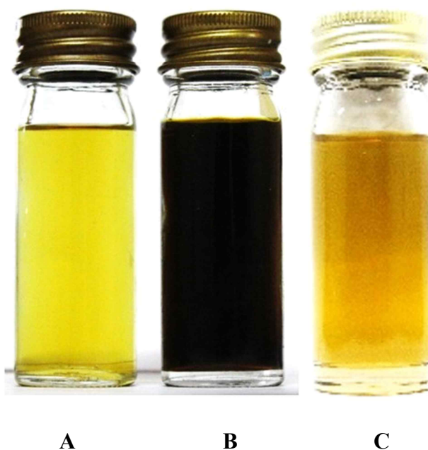
Fig. S1: (A) Garcinol dissolved in methanol, (B) G-AgNPs aqueous solution and (C) Chemically synthesized AgNPs aqueous solution.
