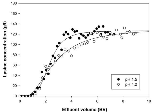
**Fig. 1.** Effluent profiles of lysine breakthrough in the cation-exchange bed. ●, Feed pH=1.5; ○, Feed pH=4.0.
