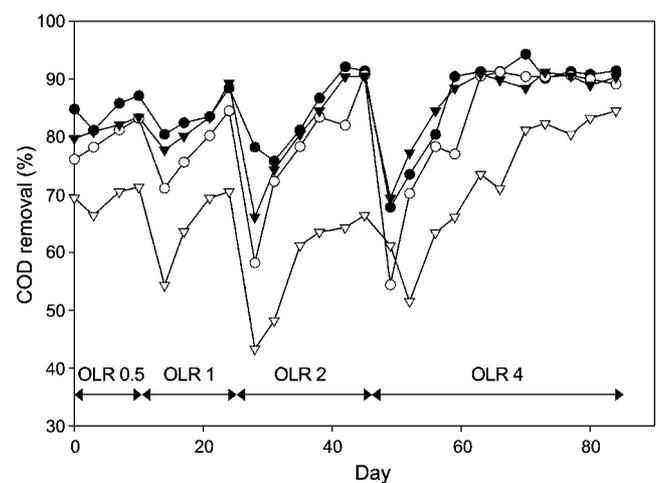
**Fig. 6.** Continuous operation of UASB reactor to treat landfill leachate and synthetic wastewater by increasing OLR (organic loading rate; kg COD/m<sup>3</sup>·day).
