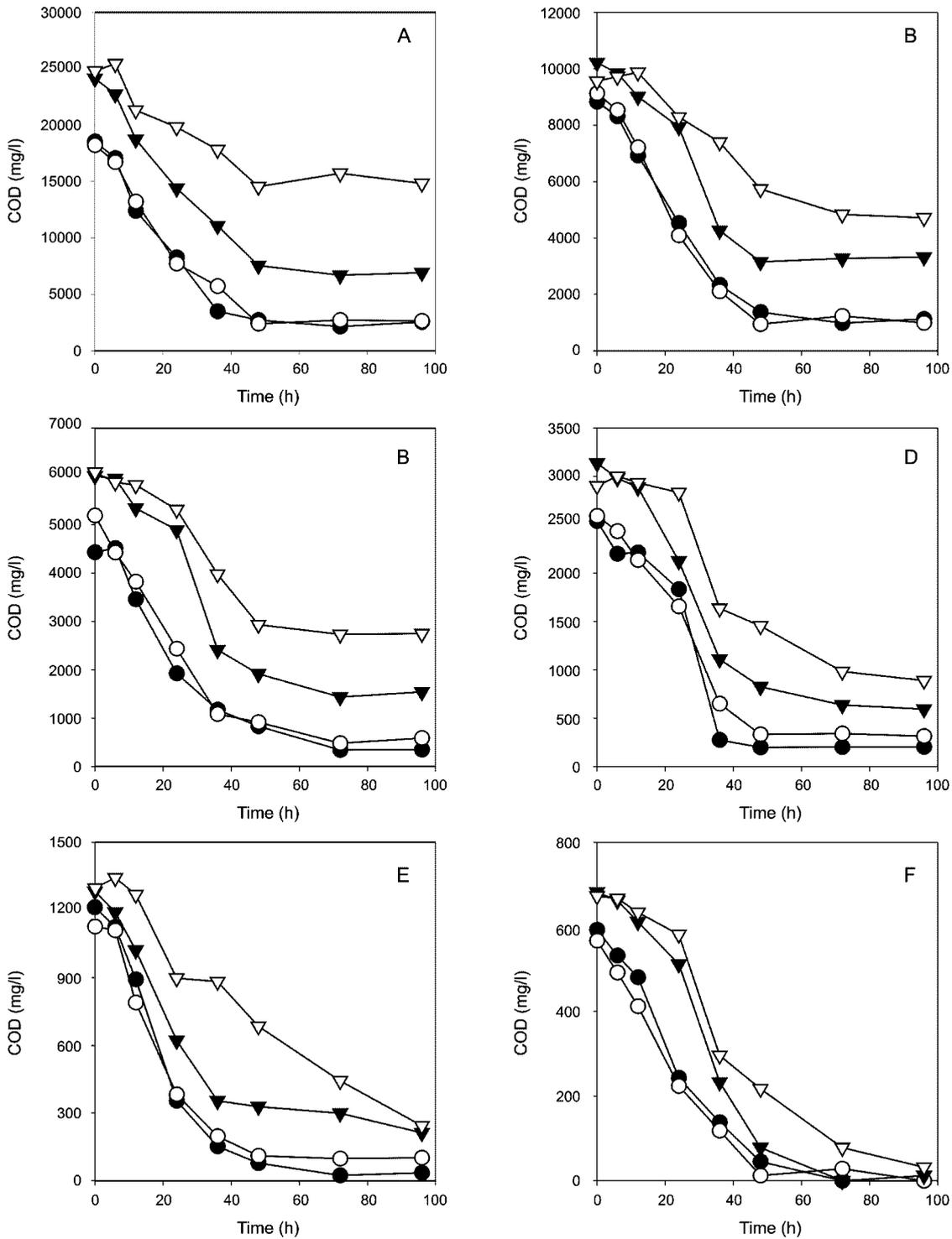
**Fig. 4.** Decrease in COD degree from landfill leachate and swine wastewater treated by intact and disintegrated granules with (A) 2<sup>0</sup>, (B) 2<sup>1</sup>, (C) 2<sup>2</sup>, (D) 2<sup>3</sup>, (E) 2<sup>4</sup>, (F) 2<sup>5</sup> dilution. (●) Swine wastewater treated by intact granules, (○) Swine wastewater treated by disintegrated granules, (▼) Landfill leachate treated by intact granules, (▽) Landfill leachate treated by disintegrated granules.
