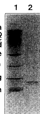
Fig. 4. Isoelectric focusing analysis of purified SOD by Mini IEF cell ((Model 111, Bio-Rad Co. U.S.A.) using 5% polyacrylamide gel and 2% ampholyte (pH 3.0 to 10.0).
